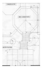
^ This construction drawing shows the arrangement of the octagonal patio, wooden steps and dry river bed
